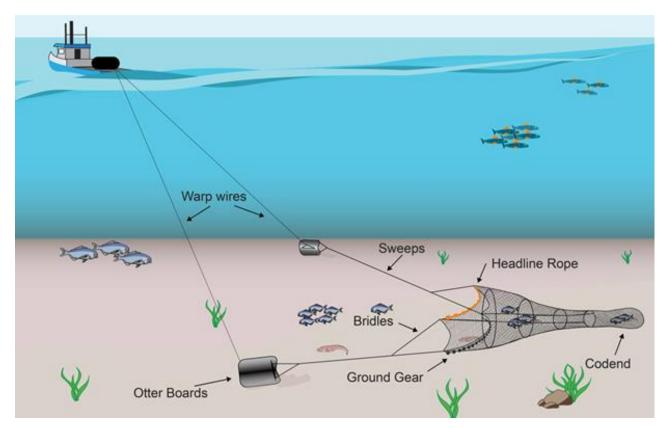
**Figure 7.** Schematic of a demersal trawl (Source: <a href="https://www.afma.gov.au/fisheries-management/methods-and-gear/trawling">https://www.afma.gov.au/fisheries-management/methods-and-gear/trawling</a>)
